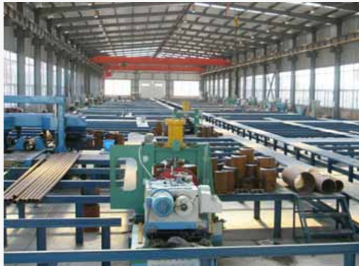
Pipe Bevel Machining Flow Line(B-type)
