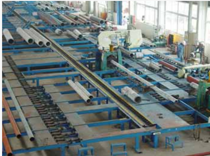
Pipe Bevel Machining Flow Line(C-type)
