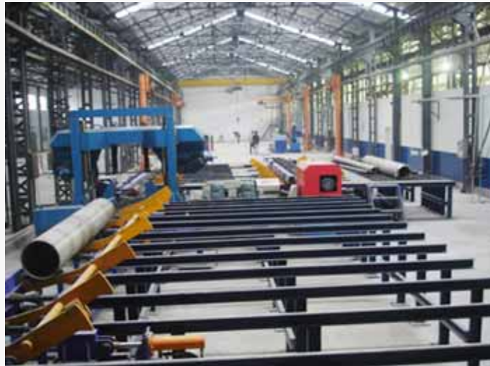
Pipe Bevel Machining Flow Line(B-type)
